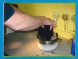
To create an ice plug, take a still inverted bot tle and place the neck into solution.
